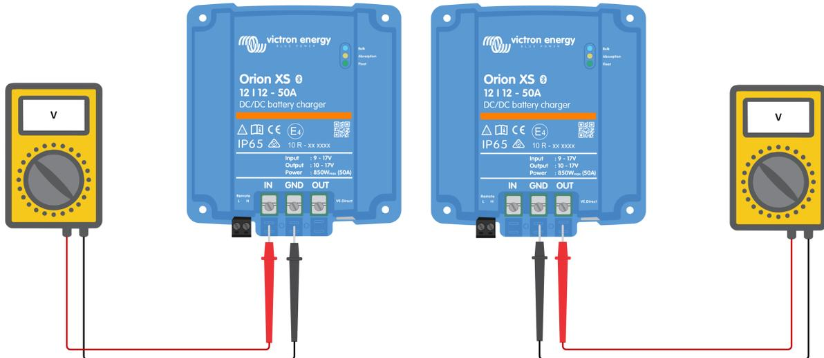
The reason for measuring the battery voltage at the charger terminals is to rule out possible problems with the wiring, fuses and/or circuit breakers in the path between the battery and the charger.
