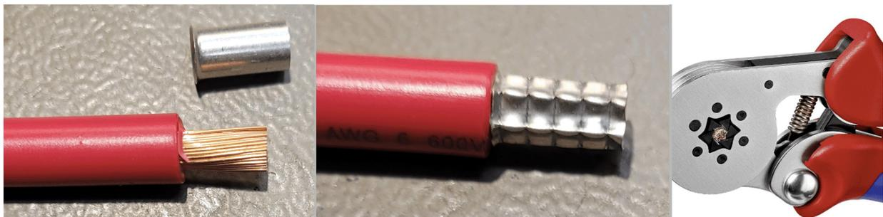
Hexagonally crimped bootlace ferrule
